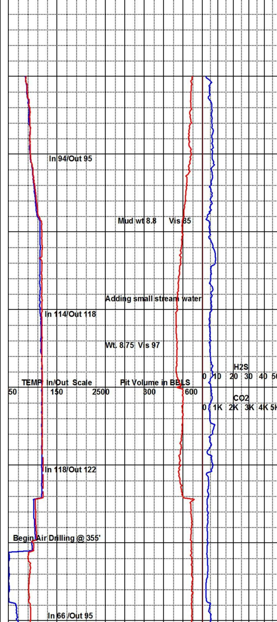
**NOTE:** Commence logging @ 8:00 hrs on 8/27/08. Hole was previously drilled with 36" bit to 50' and 30" conductor was set to 50'. Drilled out of conductor with 26" bit. All depths are referenced from 14' kelly bushing. Hole depth is determined by drillers pipe tally.
